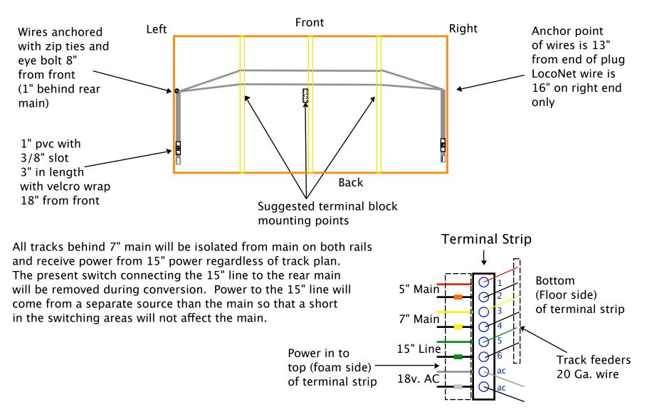
Drawing is the underside of a module
