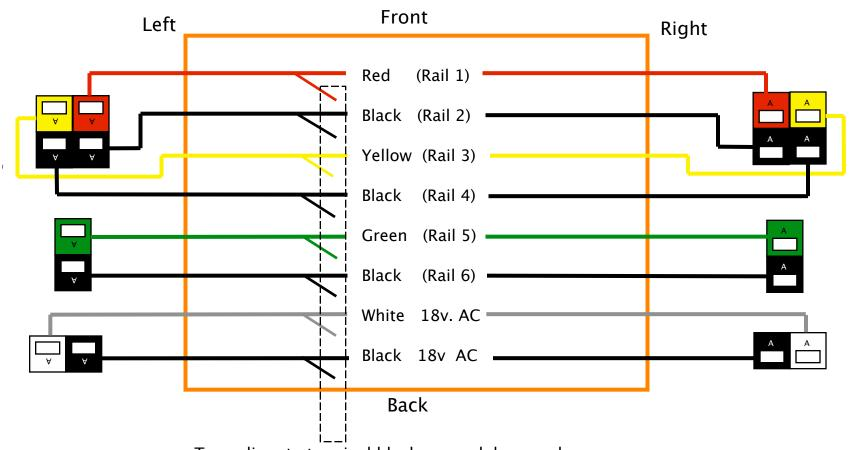
Tap splices to terminal block on module cross brace. All connections to module will be made at terminal block. Absolutely no other connections will be made to through wiring.
